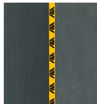
A split face slate surface treated with Fila StonePlus (left) and a untreated sample (right). It is evident that even darker colours are enhanced.
